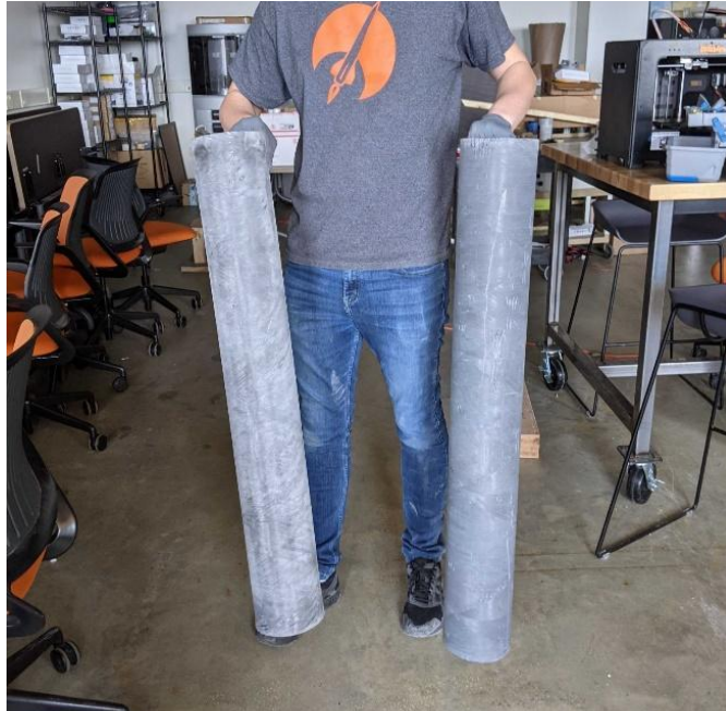
Figure 10. Carbon fibre tubes cut to length and sanded.
