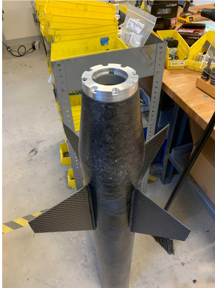
Figure 16. Assembly of the carbon fiber boattail with motor retainer
