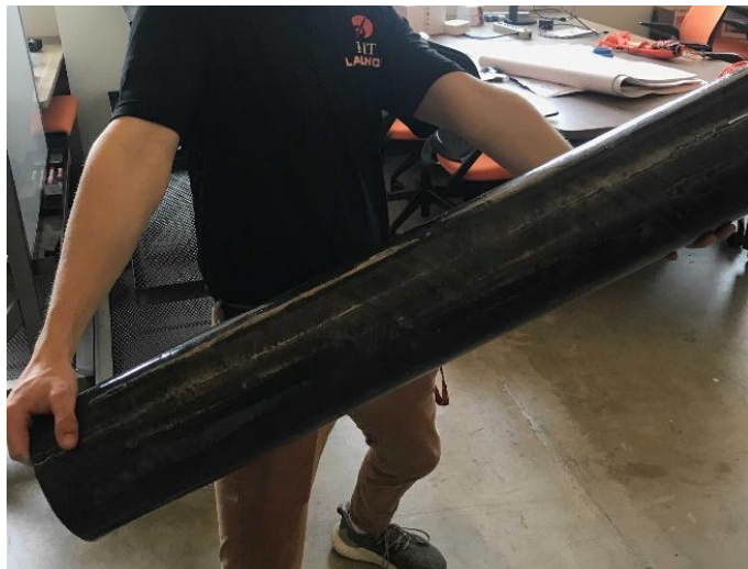
Figure 11. Final coat of polyurethane spray for a smooth finish.
