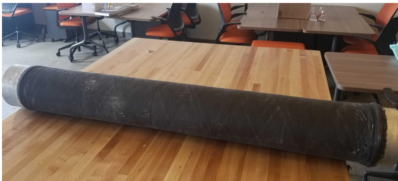
Figure 8. Carbon fiber tube after peel-ply and heat shrink have been removed.
