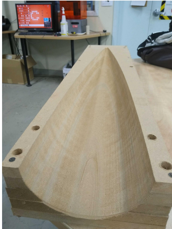
Figure 4. One half of nose cone mold routed from medium density fibreboard
