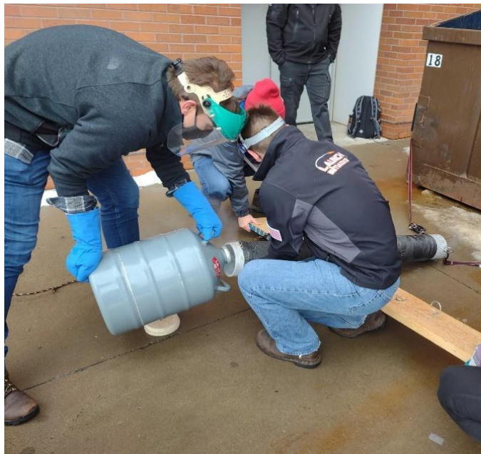
Figure 9. Pouring liquid nitrogen into the mandrel to remove the wrap.
