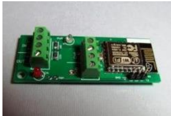
Figure 14: Eggtimer Wifi Switch for Remote Arming
